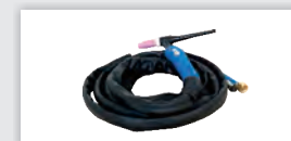
TIG torch: WP-26 Gas connector:M16 Cable length 4M 5-pin control coupler
